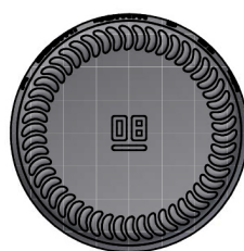
VIEW OF BASE SHOWING ALPHA NUMERIC CODE AND STANDING AREA EMBOSSED WITH STIPPLE
